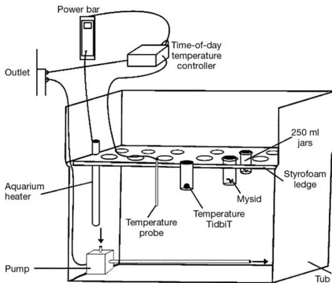
Fig. 1. Schematic of a temperature treatment tub bisected lengthways. The arrows going into and out of the pump indicate the direction of water flow
