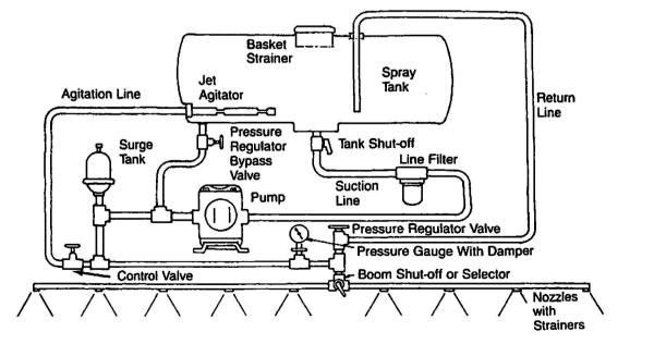
Figure 31. Components of a typical low-pressure field spray system using a diaphragm or piston pump. Roller pump would not require the surge tank.
