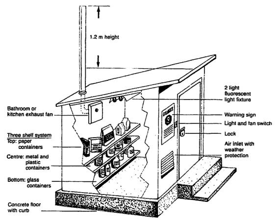
Figure 10. Layout of pesticide storage building suggested by W.C.B.
