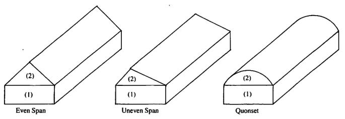
Measurements are made in metres to obtain m<sup>3</sup>. Calculate the cubic contents of the various parts as follows:
