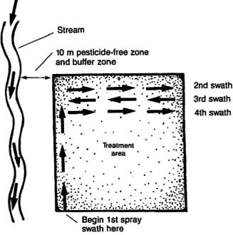
Figure 41. Suggested spray procedure to reduce drift toward the 10 m pesticide-free zone.
