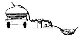
4. Backflow Preventer (in an irrigation system): is required to prevent pesticide injected into a system from flowing back into the supply line rather than out through the sprinkler heads.
