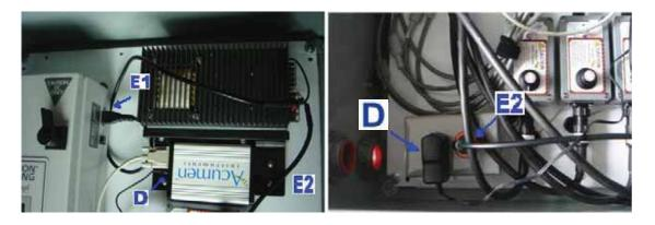
6. Connect one of the two power cords from the AC-DC power converter (black block with "radiators") to the side of the FS1001M Multiplex Transceiver System as indicated by **E1** in the previous figure. Connect the other power cord from the AC-DC power converter to a power outlet, as indicated by
