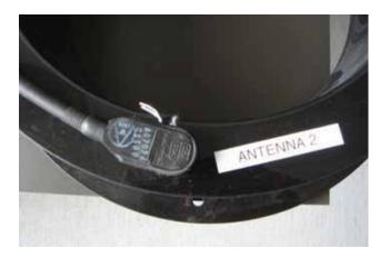
2. Pass each black antenna cable through the appropriate opening in the metal box, as shown for cable A in the figure below. Connect each cable to the corresponding tuning box (attachment located at the side of the tuning box having a black cap).
