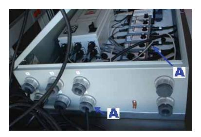
3. Attach the grey cable on the other end of each tuning box to the corresponding antenna ports on the FS1001M Multiplex Transceiver System (see cable and attachment B in the figure below). The antenna ports on the FS1001M are numbered the same way as the openings on the metal enclosure.
